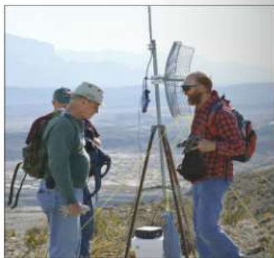
Figure 2 — From the left are Mitch, KD5HCV; Joe, KC2KG; and Alan, KESDTR, who used a compass to aim the antenna and a signal mirror to confirm the orientation. The antenna is secured with guy wires attached to 10 inch steel spikes. The cooler is to keep the battery-powered UPS warm during the night. (Paul Kinney, KD5VRU, photo)
